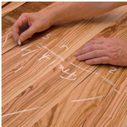
*The veneer strips are aligned and marked by the processor.*
